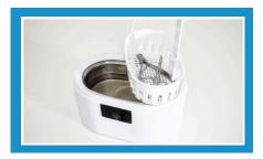
Ultrasonic cleaning works through high-frequency sound waves transmitted through liquid to scrub clean the surface of immersed items. The high-frequency sound waves (40 kHz) agitate the liquid solution of BioSON and cause the cavitation of solution molecules.
